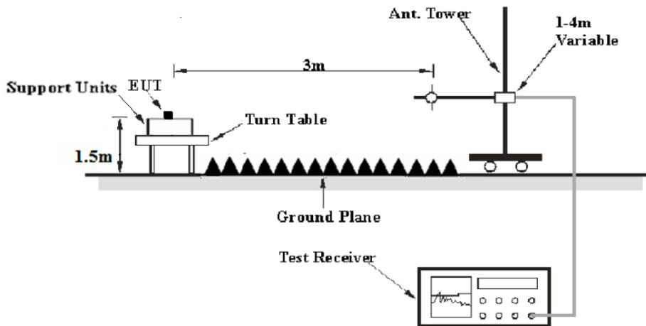
The radiated emission tests were performed in the 3 meters test site, using the setup accordance with the ANSI C63.10 - 2013. The specification used was the FCC 15 § 15.209, 15.205 and 15.231.
