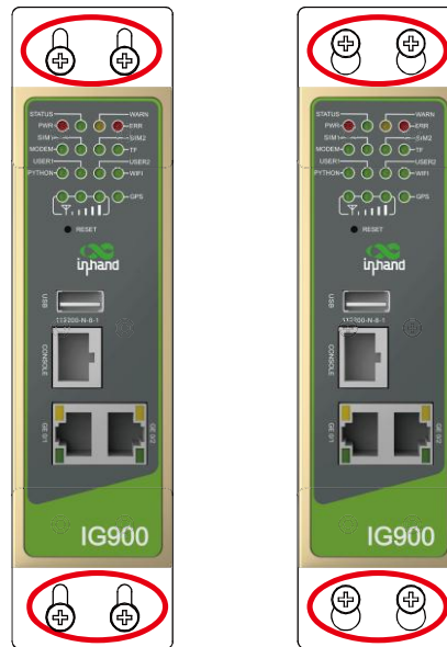
Figure 3-4 Wall mounted installation diagram
