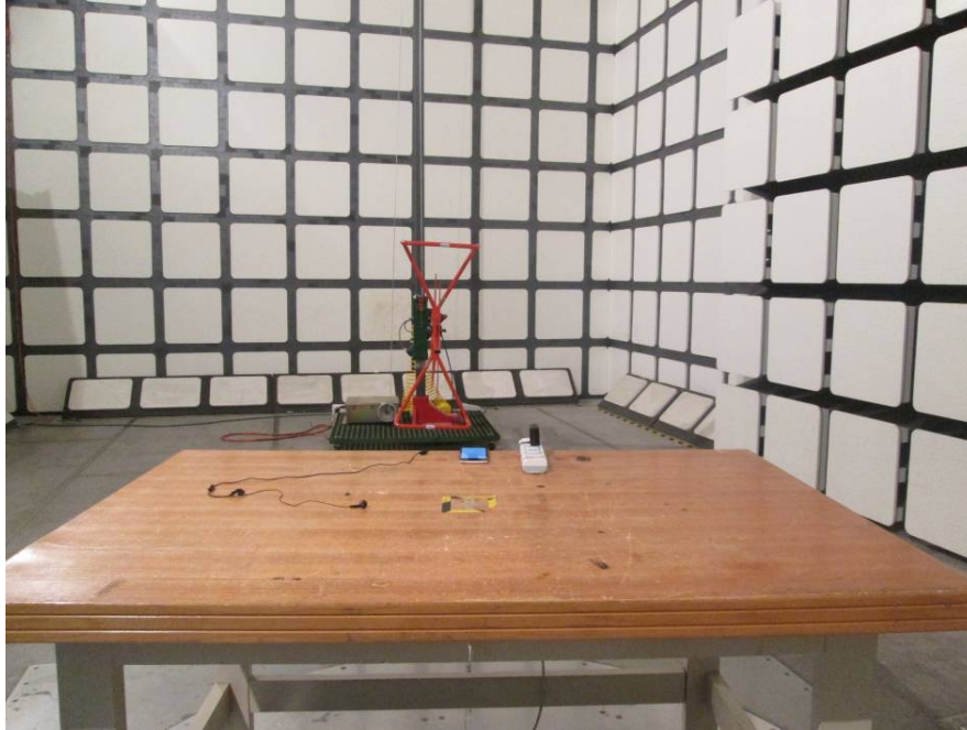
Radiated Emissions –Front View (30-1000 MHz)
