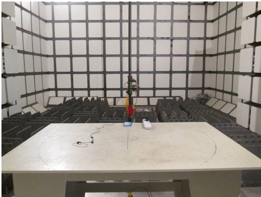
Radiated Emissions –Front View (1-25 GHz)
