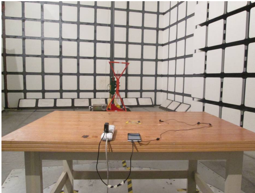
Radiated Emissions –Rear View (30-1000 MHz)
