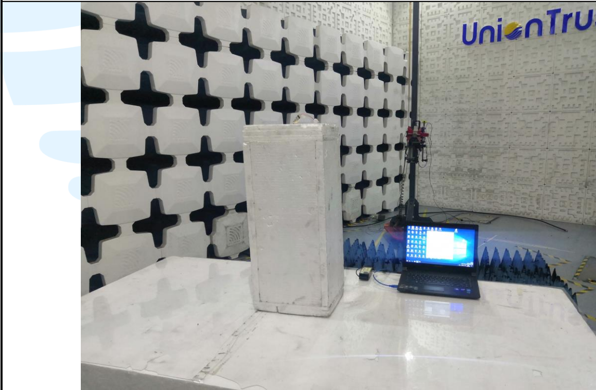
Radiated emission Test Setup (Above 1 GHz) -Right
