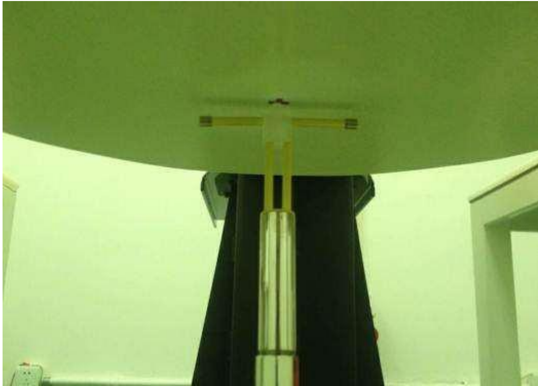
Picture 10-2 Photo of Dipole Setup
