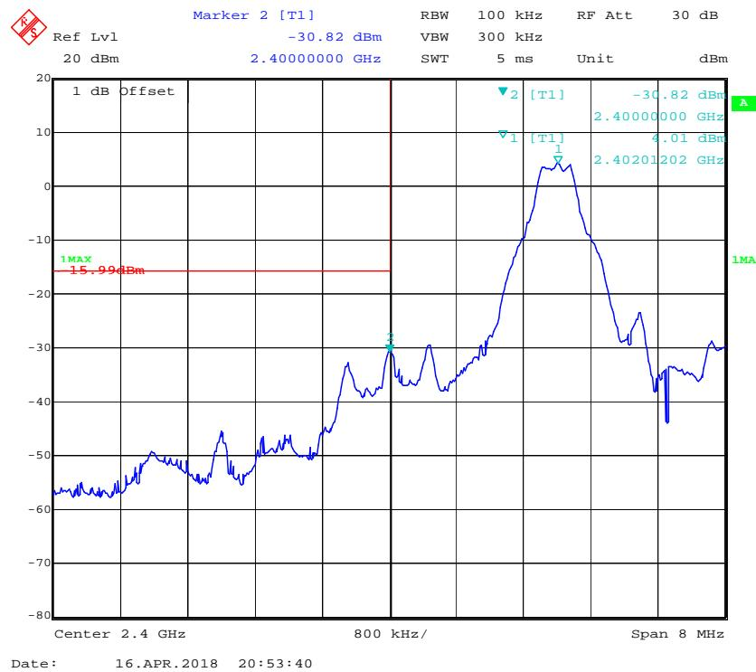
**Band Edge, Right Side**
