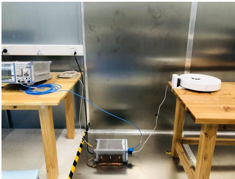
Photograph 3: Set-up photo for Conducted Emission
