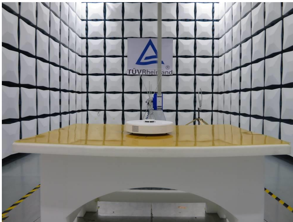
Photograph 1: Set-up photo for Radiated Spurious Emission, up to 1GHz
