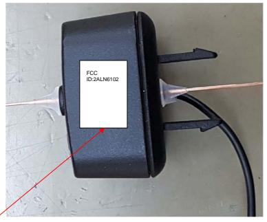
Label with **FCC ID:2ALN6102** will be located at the side of the sensor. The statement according to FCC part 15 §15.19(a)(3) is placed in User's Manual, page 3 (Application exhibit User\_manual\_29352).
