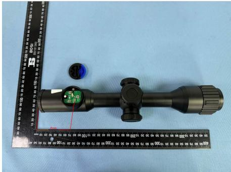
The following figure shows the shortest distance from the antenna to the extremity when the wireless function is on.
