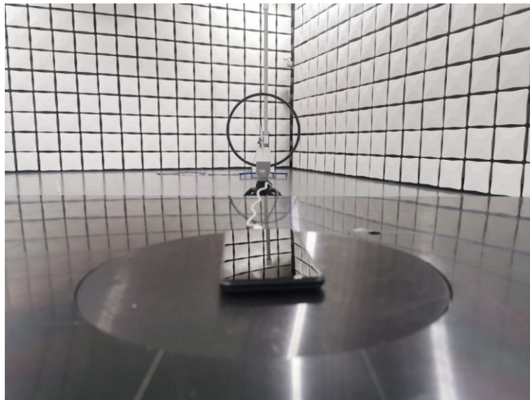
Conducted Emissions Test Setup (with charger)
