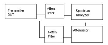
Method of Measuring Conducted Spurious Emissions
