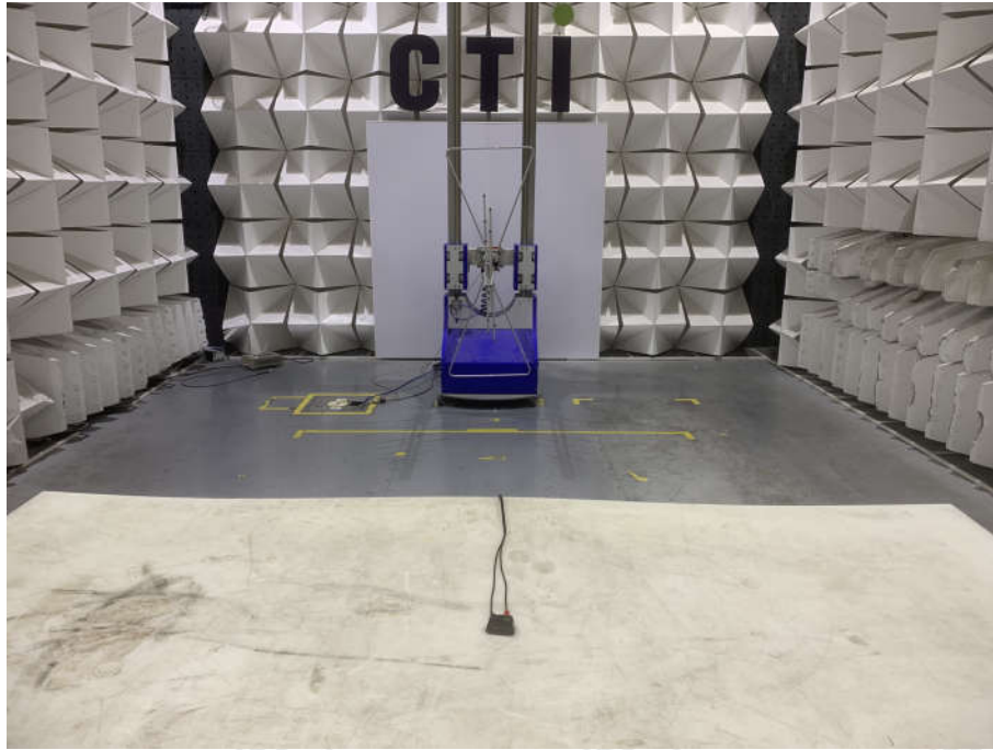
Radiated spurious emission Test Setup-1(Below 1GHz)
