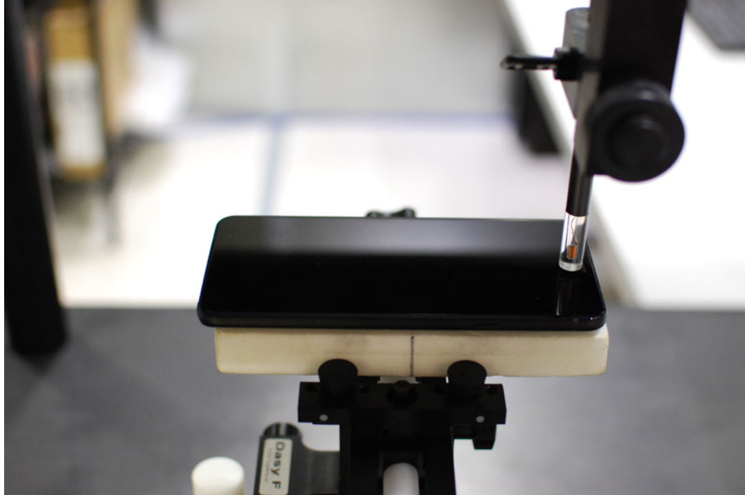
Figure 13-1 Test Setup for Wireless Device
