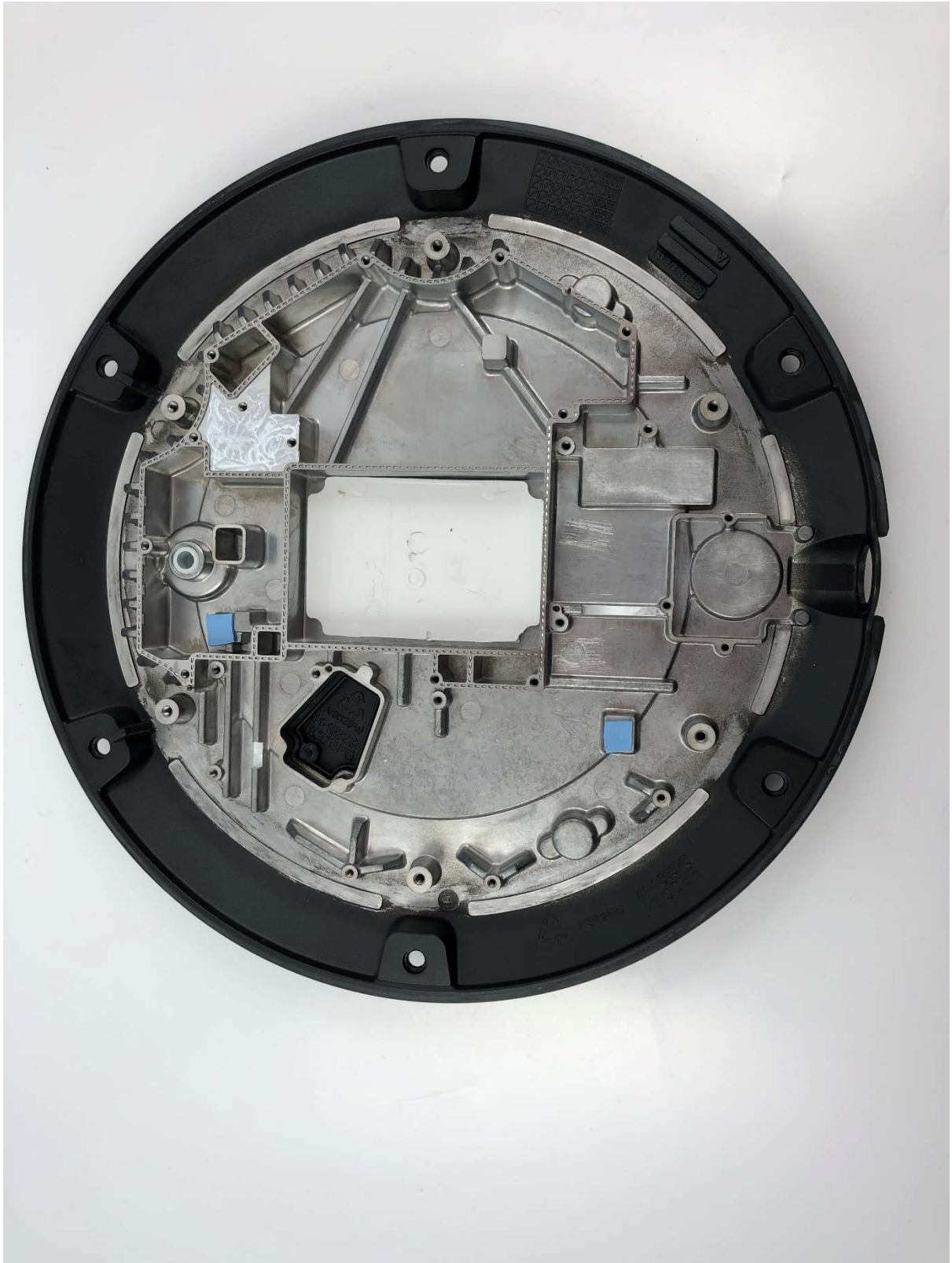
Subassembly showing a top view of bottom casing without PCBs.
