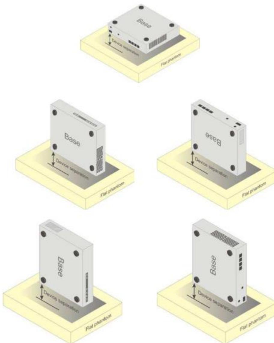
Figure 8.1 – Test positions for desktop device
