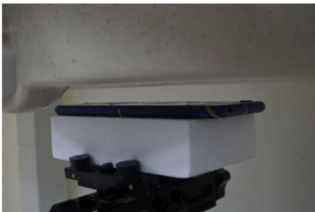
Back, Test Separation 15 mm
