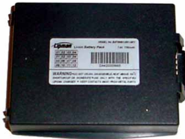
< Li-Ion battery pack (M/N: BAT09501-M01-GRY, 7.4 V, 1700 mAh) >
