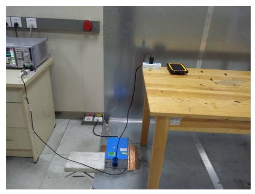
RADIATED EMISSION TEST SETUP
