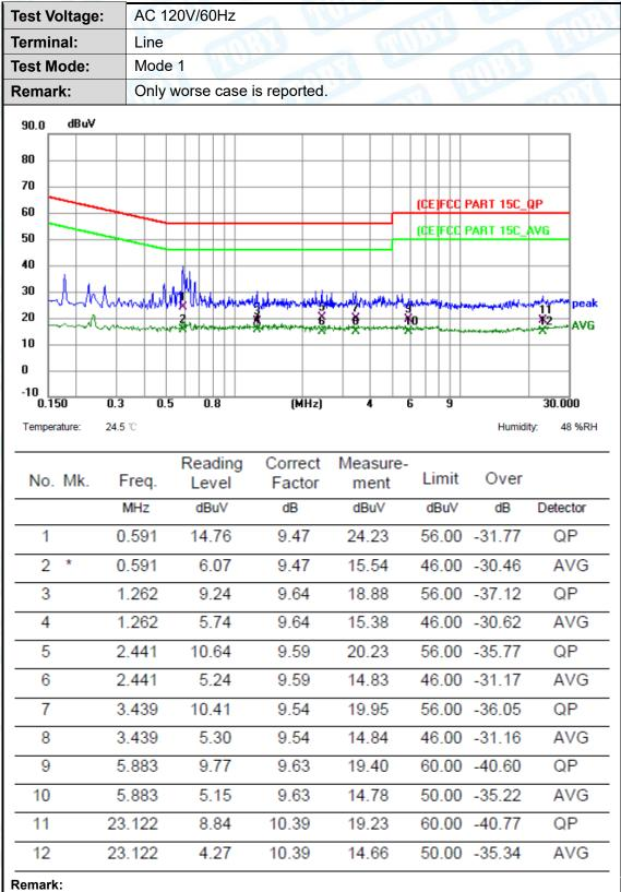
1. Corr. Factor (dB) = LISN Factor (dB) + Cable Loss (dB)
