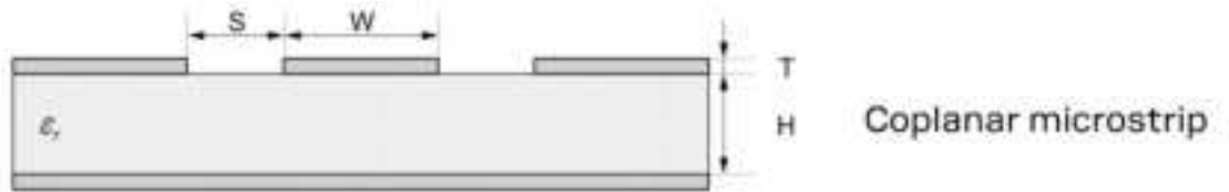
Figure 21: Coplanar micro-strip dimensions
