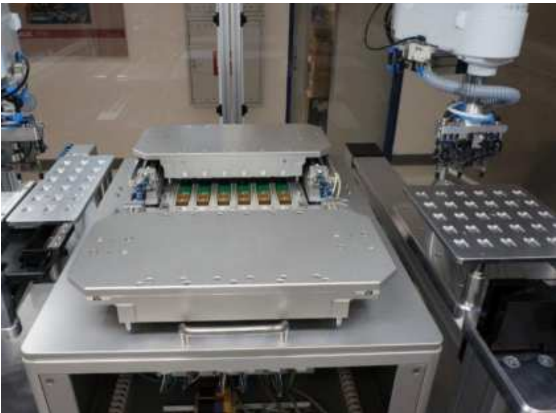
Figure 17: Automatic test equipment for module test
