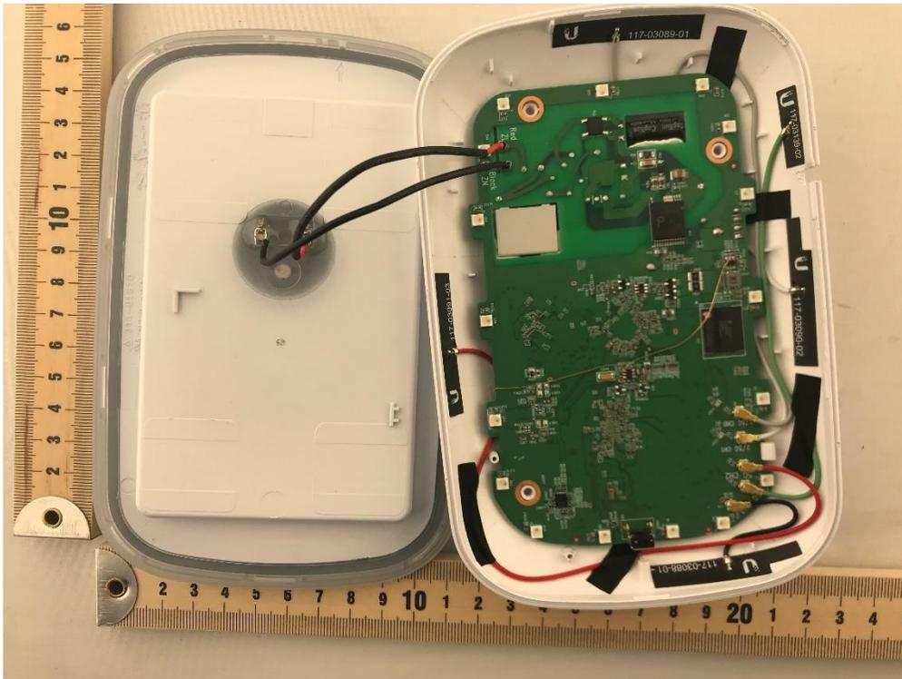
**Photograph 2: Back View of Circuit Board Without Heat Sink**
