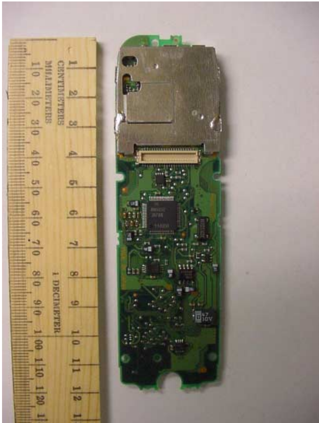
PHOTOGRAPH 10: BOTTOM OF RF PCB WITH SHIELDS
