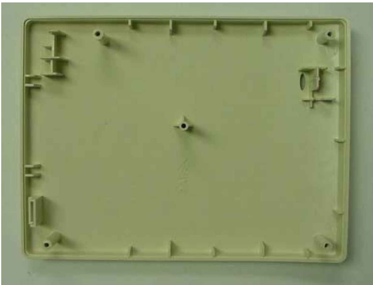
PHOTOGRAPH 14: INSIDE OF TOP COVER
