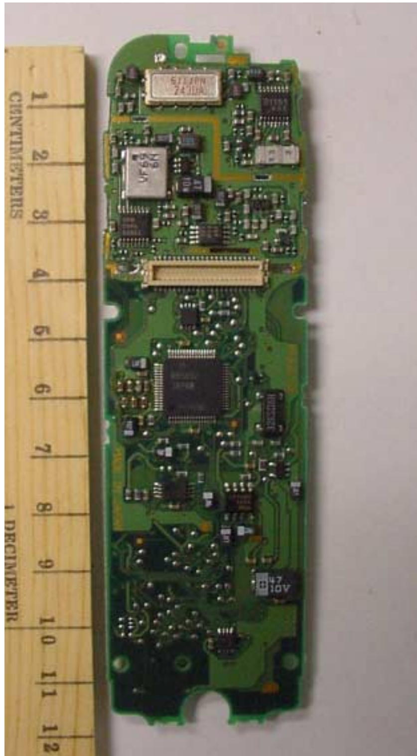
PHOTOGRAPH 11: BOTTOM OF RF PCB WITH SHIELDS REMOVED
