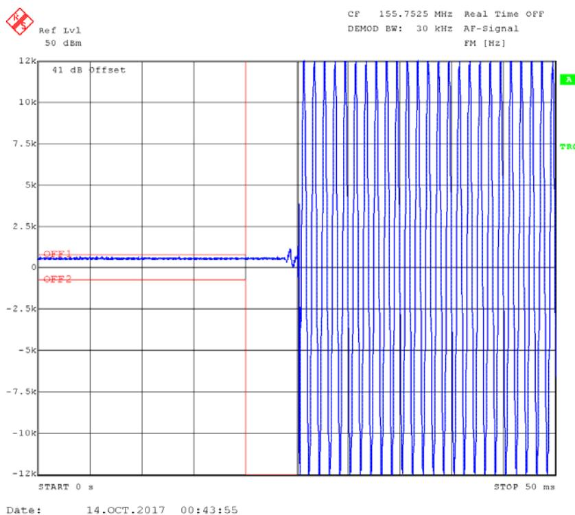
**Turn on – 155.7525 MHz, Low power level**
