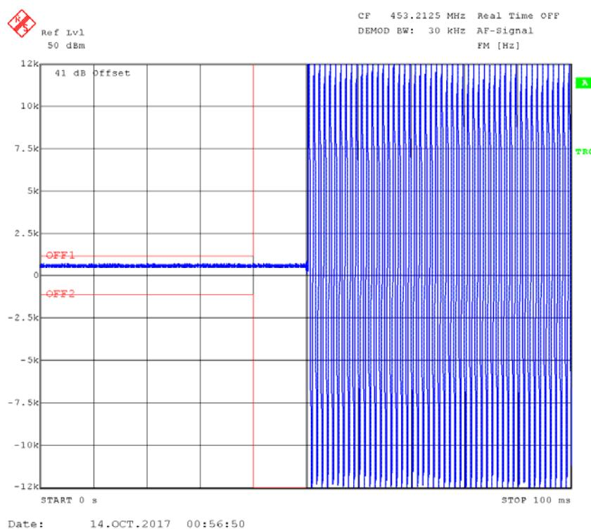
**Turn on – 453.2125 MHz, Low power level**
