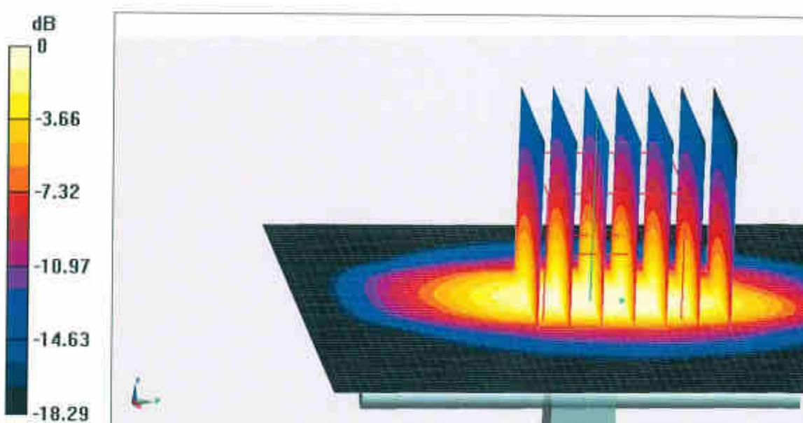
$$0 \text{ dB} = 15.6 \text{ W/kg} = 11.93 \text{ dBW/kg}$$
