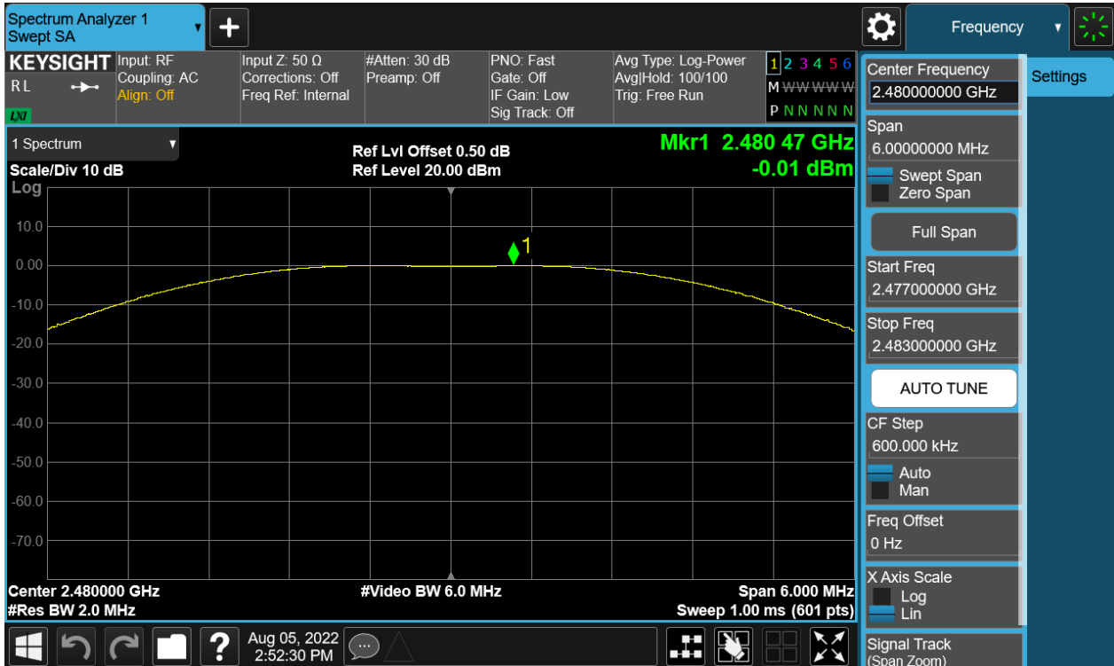
Figure 3: Peak Output Power, 2480MHz, Zigbee
