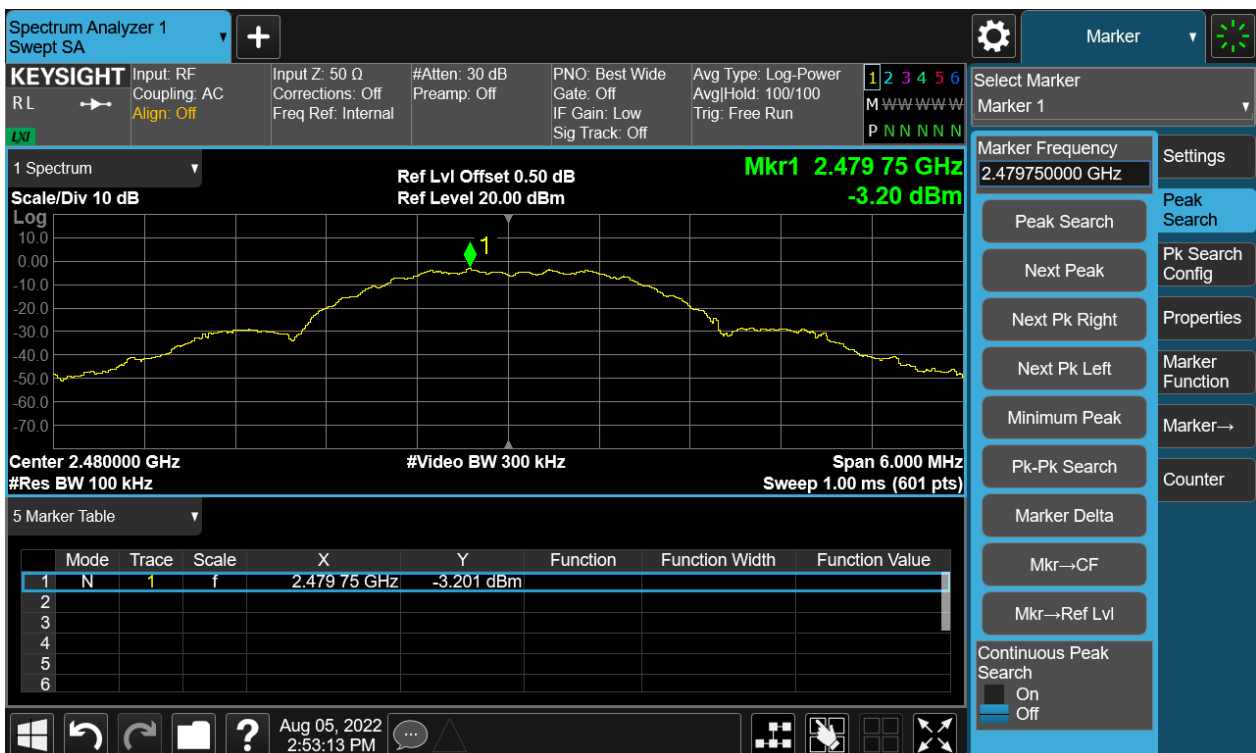
Figure 12: Conducted Spurious Emission & Authorized-band band-edge, 2480MHz, Zigbee Carrier Level
