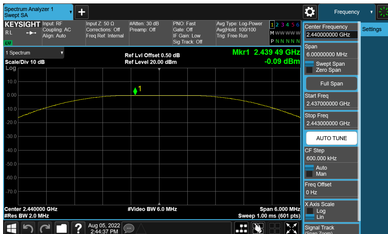
Figure 2: Peak Output Power, 2440MHz, Zigbee
