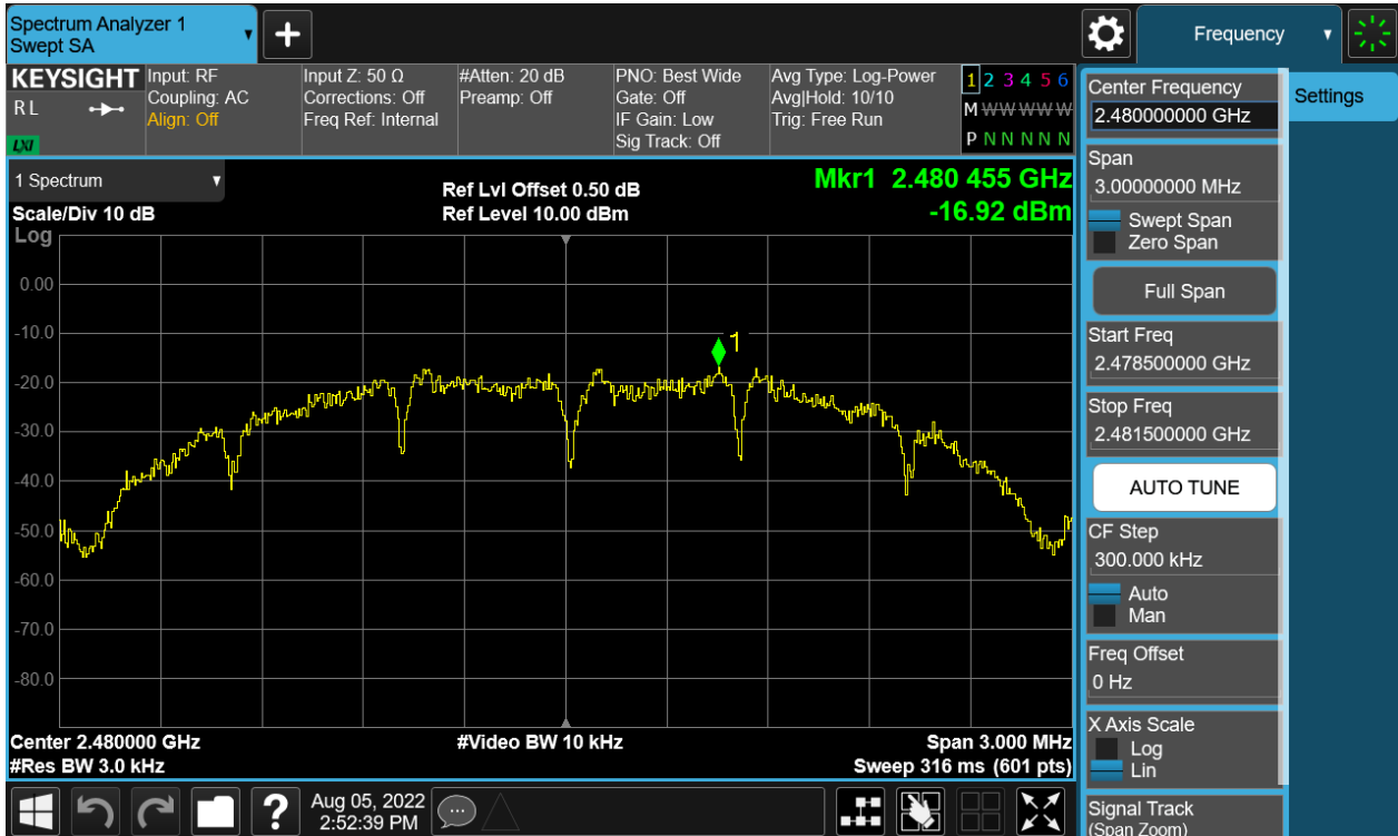
Figure 9: Power Spectral Density, 2480MHz, Zigbee
