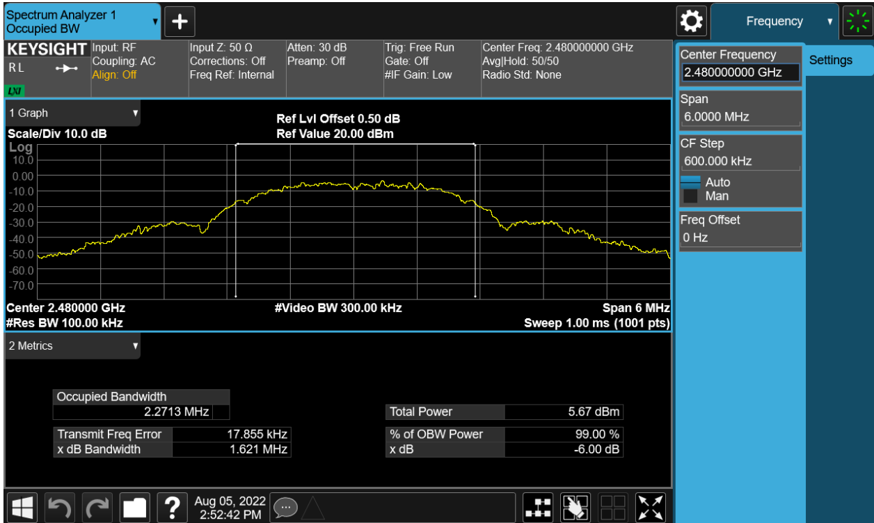
Figure 6: 6dB Bandwidth, 2480MHz, Zigbee
