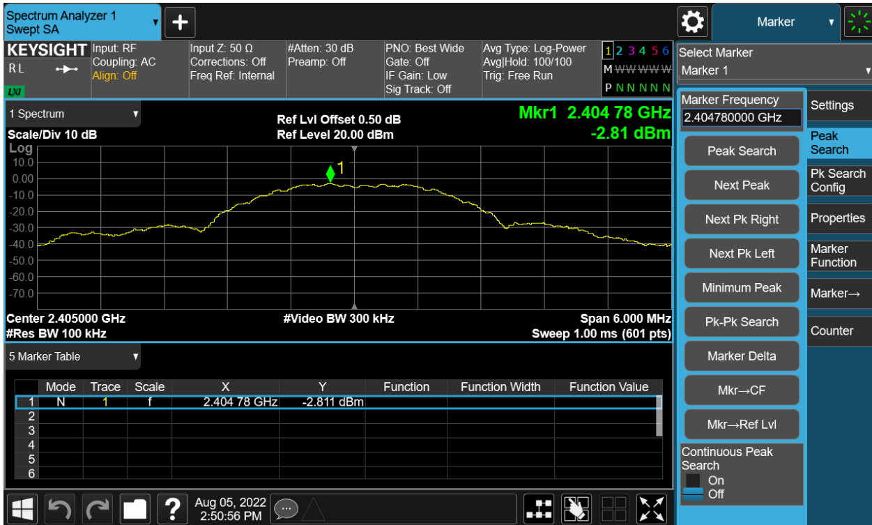
Figure 10: Conducted Spurious Emission & Authorized-band band-edge, 2405MHz, Zigbee Carrier Level
