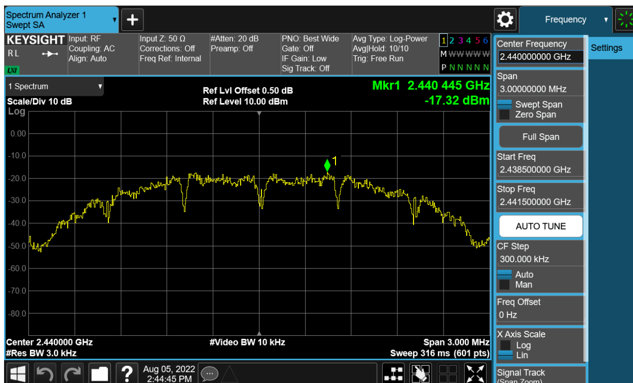
Figure 8: Power Spectral Density, 2440MHz, Zigbee
