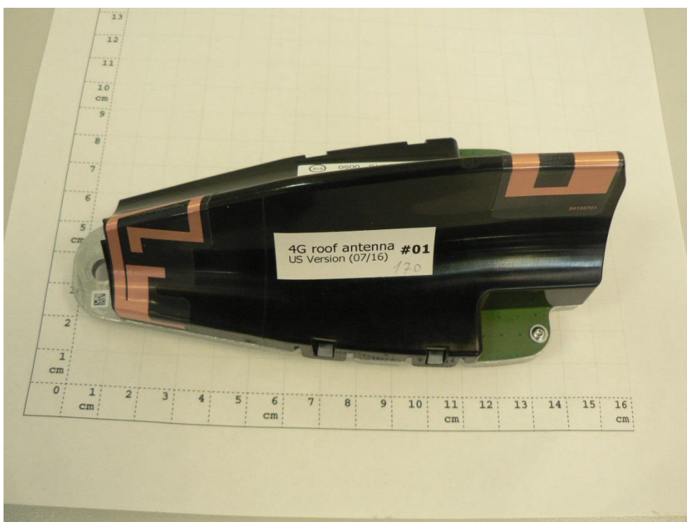
Photograph 7: Equipment under test: automotive roof pod
