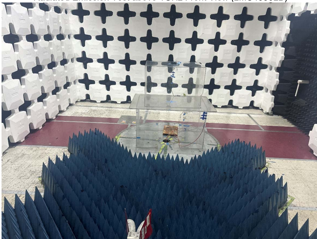
Radiated Emission Test above 1GHz Rear View (LMU4350LB)
