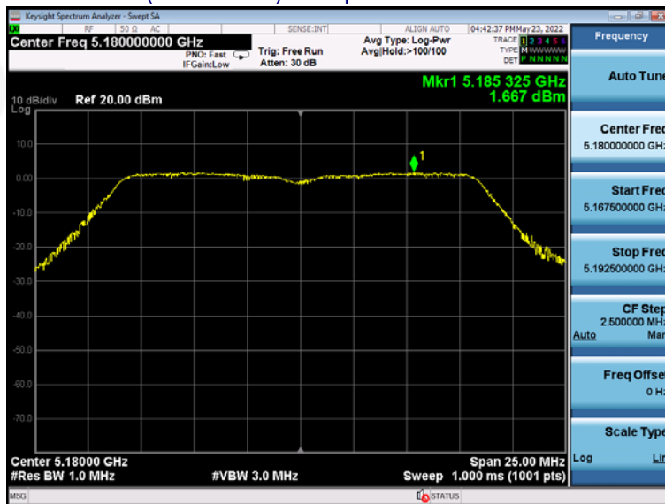
(802.11ac20) PSD plot on channel 40
