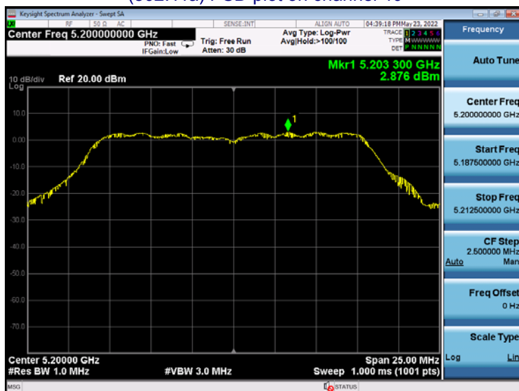
(802.11a) PSD plot on channel 48
