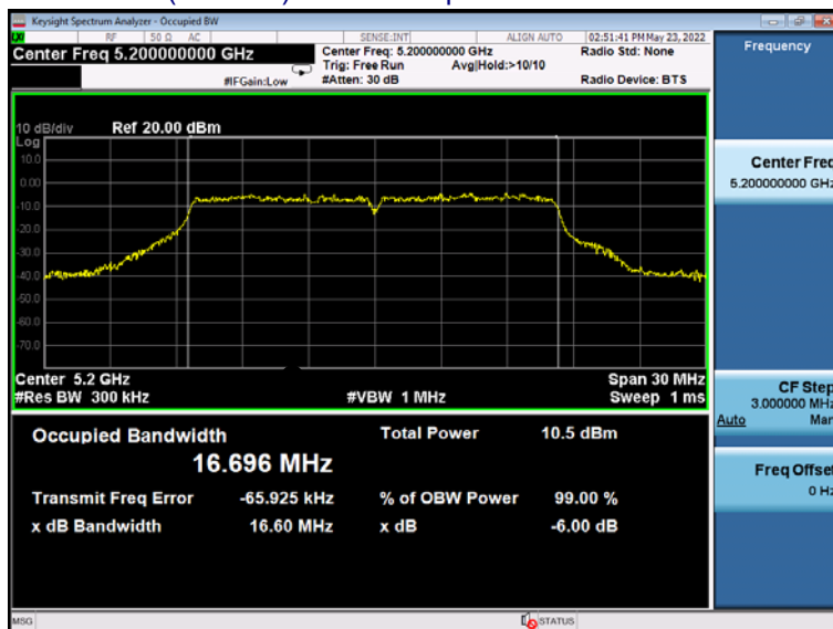
(802.11a) Bandwidth plot on channel 48
