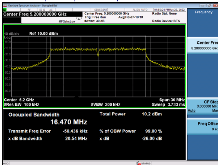
(802.11a) Bandwidth plot on channel 48
