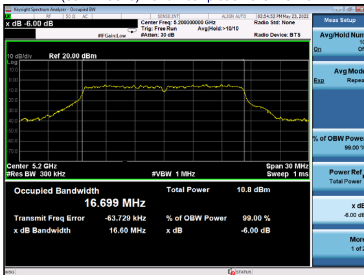
(802.11 ac20) Bandwidth plot on channel 48
