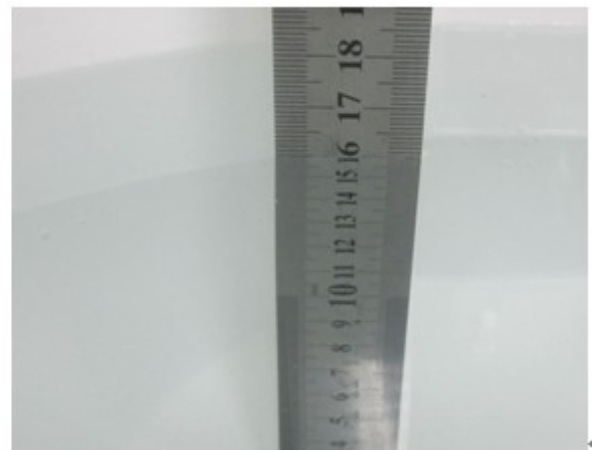
Liquid Height for Body SAR
