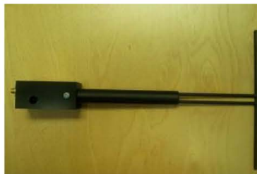
Figure 1 – MVG COMOSAR Validation Dipole
