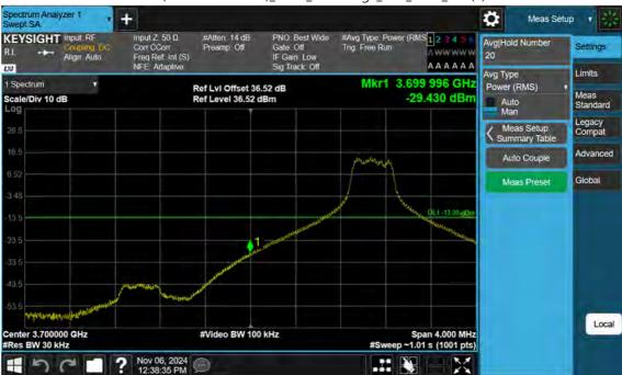
n77(3700~3980 MHz)\_90 M\_Band Edge\_Low\_BPSK\_1RB(1)
