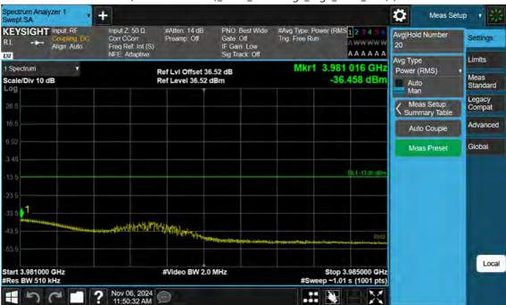
n77(3700~3980 MHz)\_60 M\_Band Edge\_High\_BPSK\_1RB(2)
