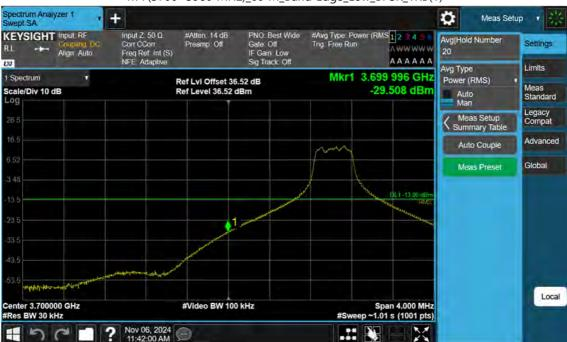
n77(3700~3980 MHz)\_60 M\_Band Edge\_Low\_BPSK\_1RB(1)
