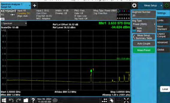
n77(3700~3980 MHz)\_70 M\_Band Edge\_Low\_BPSK\_1RB(3)
