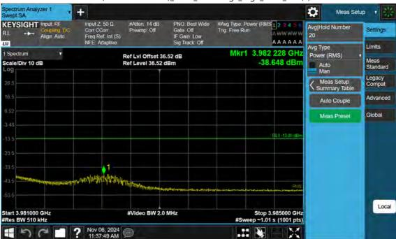
n77(3700~3980 MHz)\_50 M\_Band Edge\_High\_BPSK\_1RB(2)
