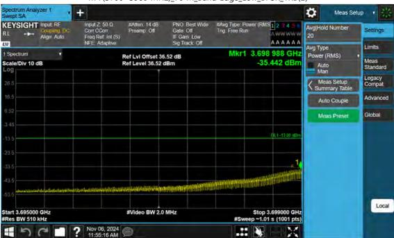
n77(3700~3980 MHz)\_70 M\_Band Edge\_Low\_BPSK\_1RB(2)
