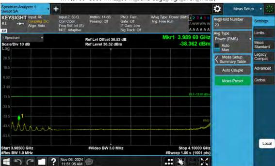
n77(3700~3980 MHz)\_60 M\_Band Edge\_High\_BPSK\_1RB(3)
