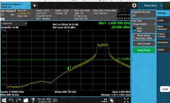
n77(3700~3980 MHz)\_80 M\_Band Edge\_Low\_BPSK\_1RB(1)
