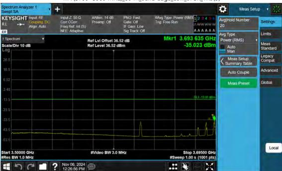
n77(3700~3980 MHz)\_80 M\_Band Edge\_Low\_BPSK\_1RB(3)
