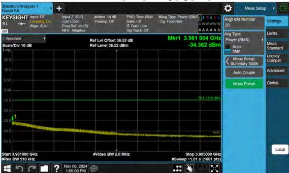
n77(3700~3980 MHz)\_100 M\_Band Edge\_High\_BPSK\_1RB(2)
