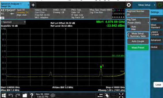
n77(3700~3980 MHz)\_100 M\_Band Edge\_High\_BPSK\_1RB(3)
