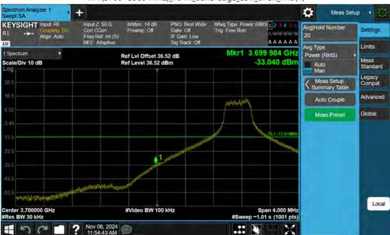
n77(3700~3980 MHz)\_70 M\_Band Edge\_Low\_BPSK\_1RB(1)
