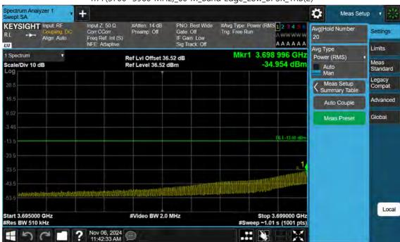
n77(3700~3980 MHz)\_60 M\_Band Edge\_Low\_BPSK\_1RB(2)
