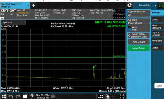
n77(3700~3980 MHz)\_60 M\_Band Edge\_Low\_BPSK\_1RB(3)
