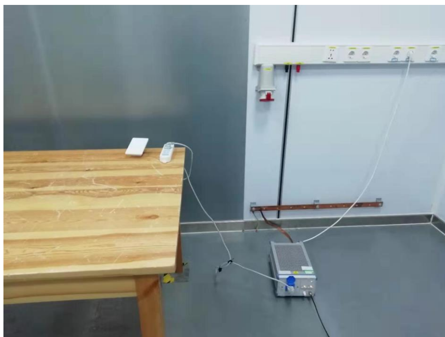
Fig. 4 Power line conducted emission setup photo
