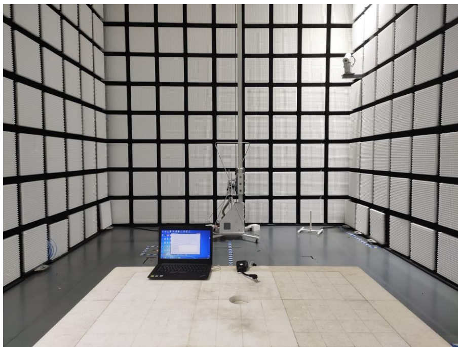
Fig. 1 Radiated emission setup photo(30MHz-1GHz)
