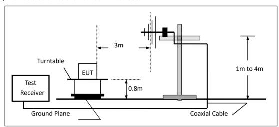
(c) For radiated emissions above 1000MHz
