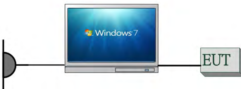
Fig. 2-2 Conducted (Antenna Port) Configuration Emission
