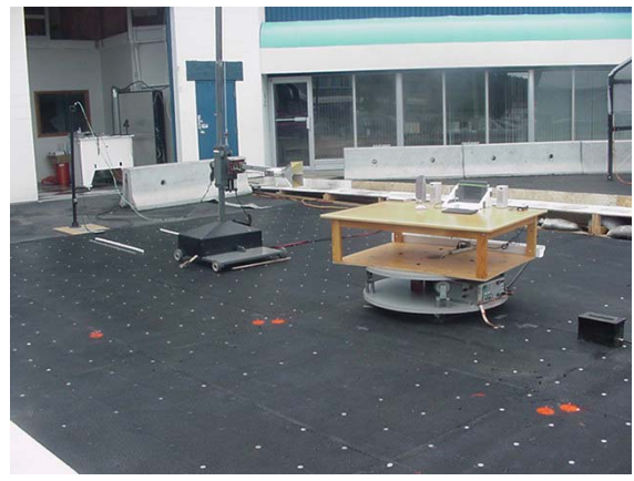
Photograph F-4 - 3115 Horn with LNA/Filter @ 1m
