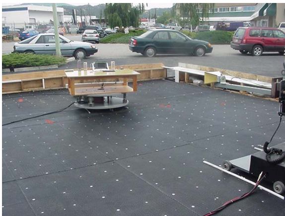
Photograph F-5 - Waveline Horn with LNA @ 1m
