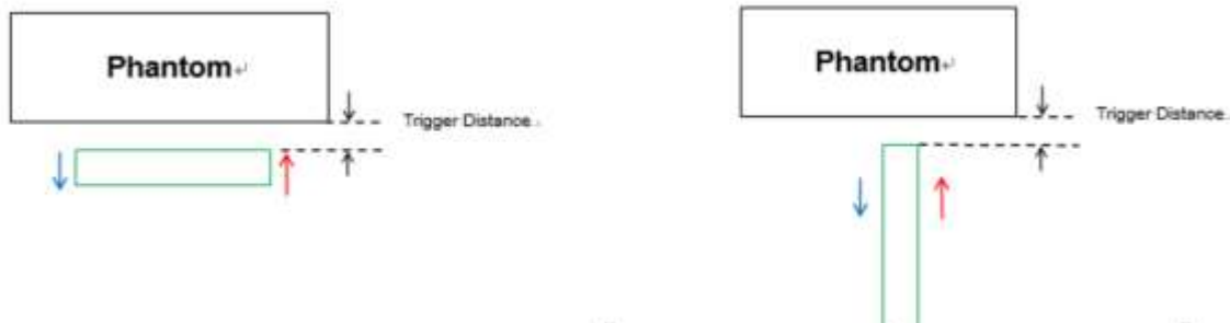
Proximity Sensor Trigger Distance Assessment KDB 616217 D04 §6.2 (Rear / Bottom / Left side)
