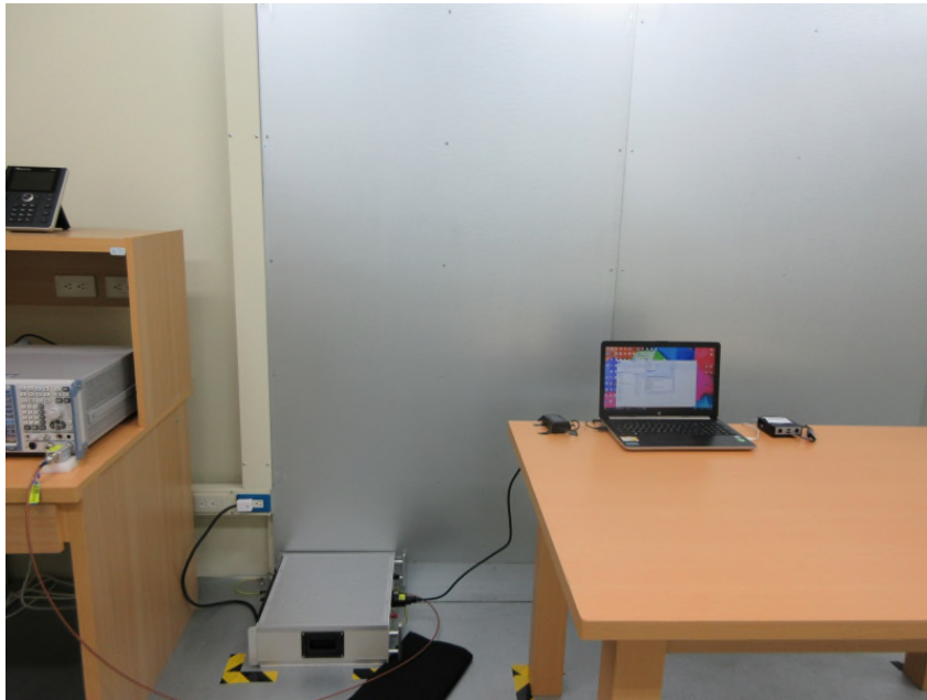
Photograph 7: Set-up for AC Mains (Front View)
