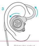
Rotate the earbud into ear canal and bend the memory wire to desired position.
