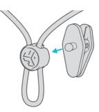
Insert the optional cable clip to the back of the cable holder.
