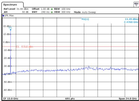
Remark: Testing is carried out with frequency rang 30MHz to 25GHz, which above 12.75GHz are attenuated more than 20dB below the permissible limits or the field strength is too small to be measured.
