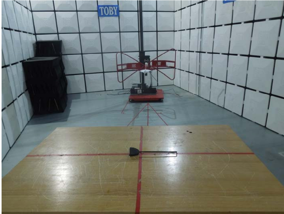
Photo of Setup for Radiated Emission (Below 1 GHz) -10 inch Ant.
