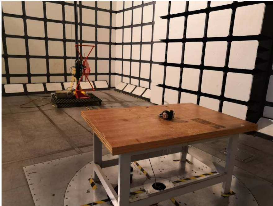
Radiated Emissions View (Below 1 GHz)
