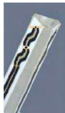
Figure 2.3 Probe Thick-Film Technique
