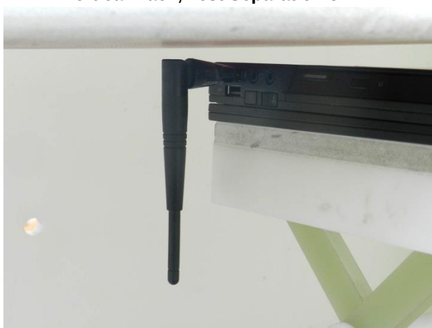
Tip Mode for Configuration 2, Test Separation 5 mm
