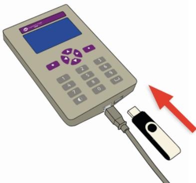
Insert the USB memory stick into the hand-held terminal and select a job following the same procedure as above.
