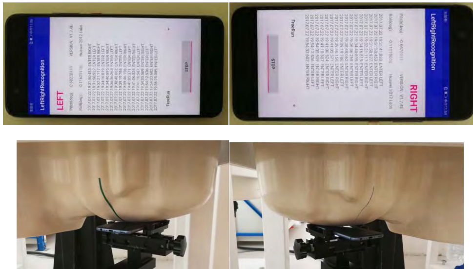
Fig 5.3.11-5 Test setup for left and right Head test Scenario
