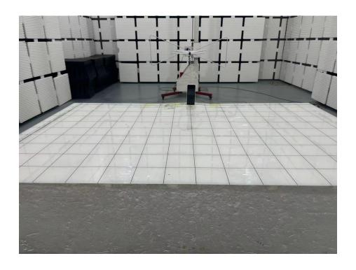
Set-up for Radiated Spurious Emission, Above 1GHz
