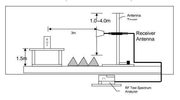
Test setup of radiated emissions above 1GHz
