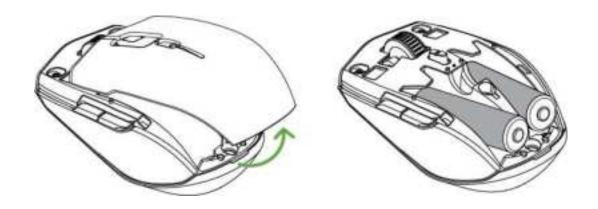
Caution: The two included AA batteries are non-rechargeable. Dispose of these batteries in accordance with your local environmental laws. For your safety, use only alkaline batteries and don't mix old batteries with new ones.
