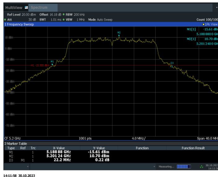
Fig.2 26dB Emission Bandwidth (802.11a, 5200MHz)
