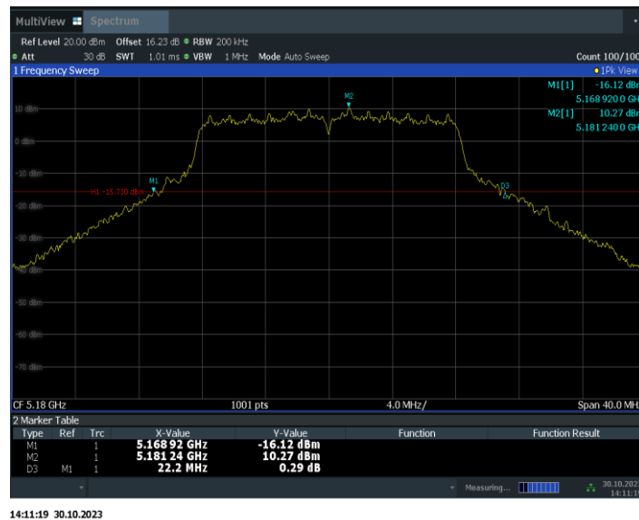
Fig.1 26dB Emission Bandwidth (802.11a, 5180MHz)
